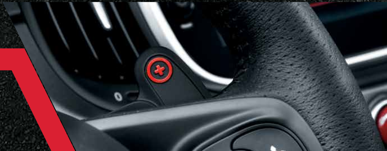
Sequential robotised gearbox with shift paddles.
