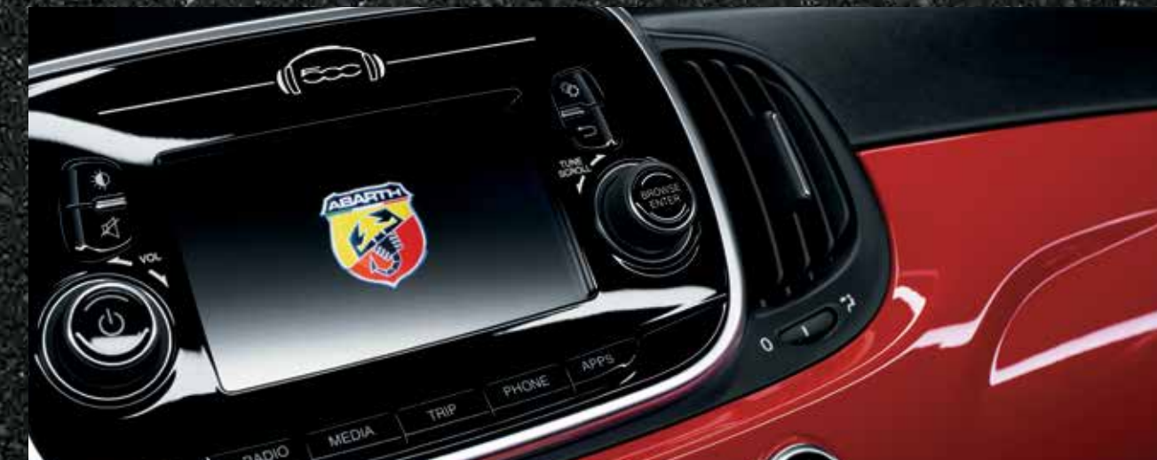
Uconnect™ radio 5" touch, Bluetooth® with 6 speakers, audio streaming and USB/AUX sockets.
